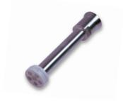
The Bio Coupon assembly is a simple device for monitoring bacterial activity. The Bio Coupon assemblies comprises of a housing with 5 Coupons directly exposed to the internal environment in a pipe or vessel.
