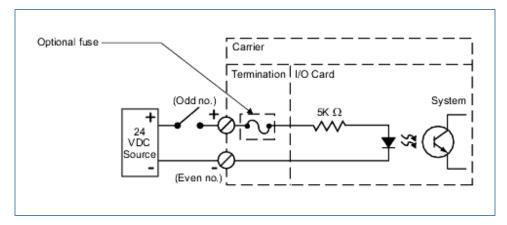
Simplified circuit and connection diagram for DI card, 8-channel, 24V DC, Isolated.
