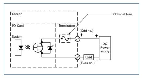
Simplified circuit and connection diagram for DO card, 8-channel, 24V DC, Isolated.
