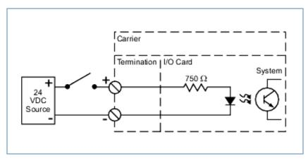
Simplified circuit and connection diagram for PCI card, 4 channel, 24V DC, Isolated.
