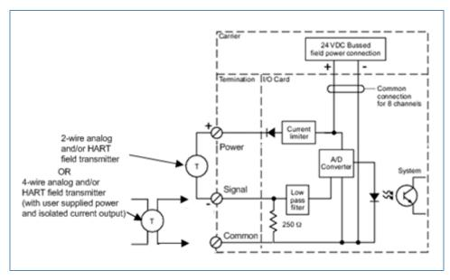
Simplified circuit and connection diagram for AI card, 8-channel, 4 to 20 mA, HART.
