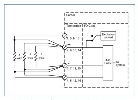
Simplified circuit diagram of Isolated Input card, RTD, 4 channels.
