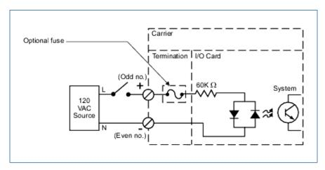
Simplified circuit and connection diagram for DI card, 8-channel, 120V AC, Isolated.
