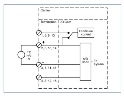
Simplified circuit diagram of Isolated Input card, Thermocouple, mV, V, 4 channels.
