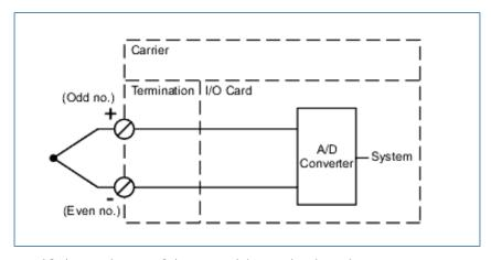
Simplified circuit diagram of Thermocouple/mV card, 8 channels.
