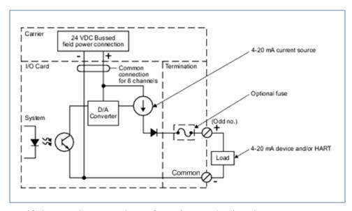
Simplified circuit and connection diagram for simplex AO card, 8-channel, 4 to 20 mA, HART.
