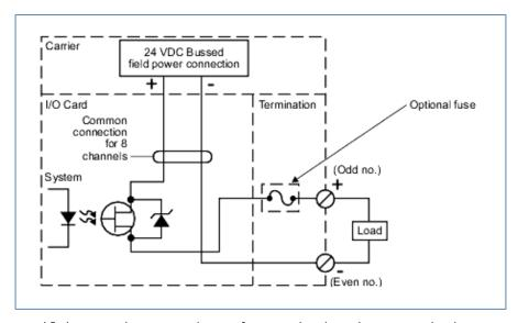
Simplified circuit and connection diagram for DO card, 8-channel, 24V DC, High Side.
