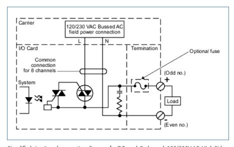
Simplified circuit and connection diagram for DO card, 8-channel, 120/230V AC, High Side.
