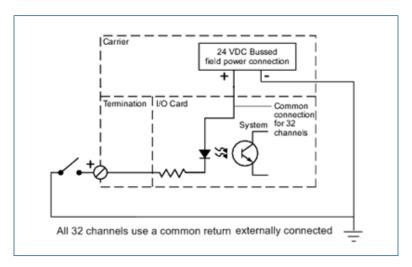
Simplified circuit and connection diagram for DI Card, 32-channel, 24V DC, Dry contact.
