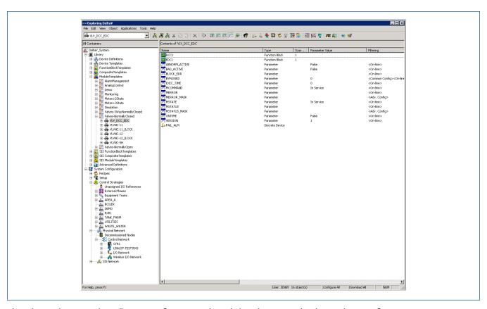
The DeltaV Explorer centralizes all system configuration tasks, including alarm, control and smart device configuration.
