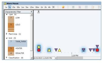
Alarm with common characteristics are automatically identified, enabling the operator to more easily comprehend the overall situation.
