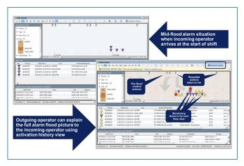
Shift transitions represent a critical moment, especially if an alarm flood is in progress. The Alarm Mosaic Activation History View allows the incoming operator to observe alarms and control actions from the prior shift.
