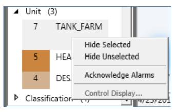
With a single mouse-click the operator can mass acknowledge, filter out, or select only the alarms with a shared characteristic.
