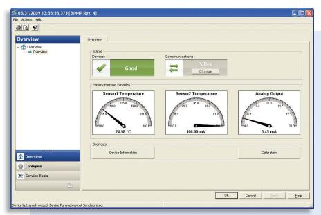
Fig. 1. In the basic structure for the new graphical interface, application of human centered design principles led to screen displays that provide information on 80% of the most common tasks performed by technicians in the field. These displays tell if a device is working (or not), if alerts are present and if the device is communicating and providing access to calibration functions, with no confusing technical jargon to interpret.
