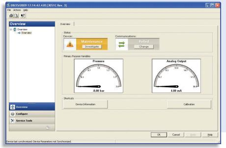
Fig. 2. If there is a problem, the word "Maintenance" appears in the "Device" box, along with a button for further evaluation. This will provide guidance for further action to determine the nature of the problem and if repair or replacement is necessary. A pop-up window leads to problem-solving instructions.
