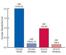
**Figure 1.** The average number of signals transmitted per second by measuring devices in two closed-loop scenarios, alongside integrated absolute error (IAE) values. Wireless devices measuring a flow-control variable using the reportby-exception communications scheme transmit about one-tenth as many signals as wired devices using the standard scheme. While measuring a pressurecontrol variable, report-by-exception transmits about one-sixth as many signals. IAE is comparable in both scenarios.
