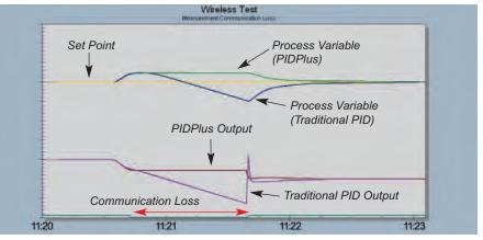
**Figure 3:** Simulation of a process disturbance, with controller input interrupted by a loss of communications. Note that in a real-life situation, process variable data would not be available for the entire period.
