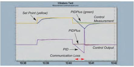
**Figure 4.** PIDPlus and traditional PID respond to a set-point change followed by interrupted wireless measurement updates. Note that in a real-life situation, process-value data would not be available during communication interruptions.
