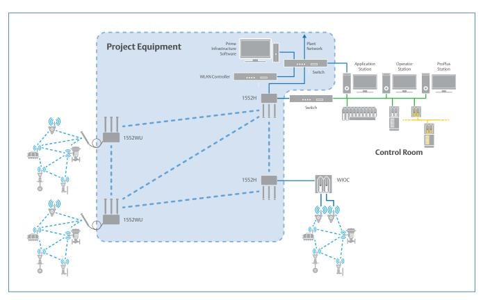
Example of a Wireless Field Data Backhaul solution architecture.
