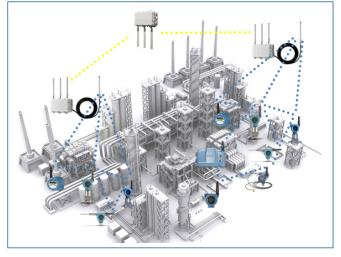
An Emerson Smart Wireless Field Data Backhaul Solution integrates WirelessHART data from remote areas of your plant.
