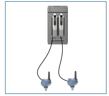
Wireless I/O Card connected to Field Links.
