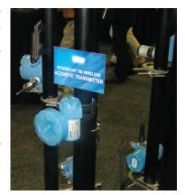
In steam trap monitoring, a wireless acoustic transmitter 'listens' for ultrasonic noise created by steam or condensate, and also measures the temperature at the steam trap inlet via a built-in sensor.
