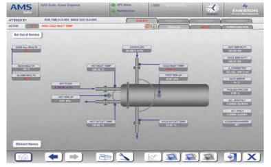
Wireless temperature monitoring enables valuable information on heat exchanger condition and performance.
