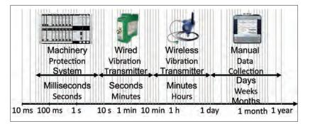
*Figure 1: Frequent data collection to catch developing issues early requires automation.*
