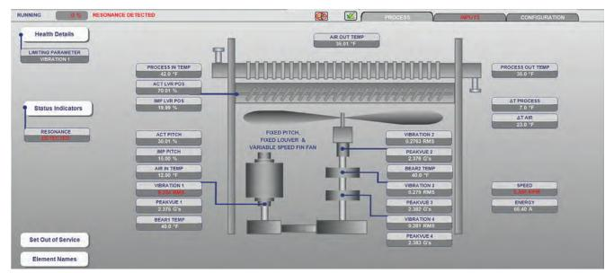
Figure 4: ACHE display – resonance alarm.
