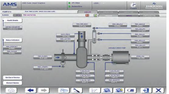
Figure 5: Pump display – pressure instability alarm.
