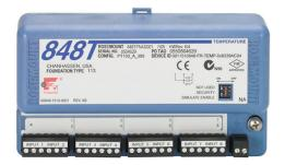
The Rosemount 848T offers a low-cost solution for high density measurements. The transmitter accepts eight independently configurable sensor inputs, and can be mounted close to the process to improve data quality. FOUNDATION Fieldbus architecture allows up to 128 temperature measurements to be transmitted on a single H1 Fieldbus line.
