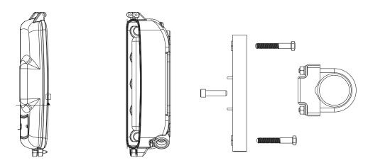
Figure 11: Mount stainless steel on vertical pipe
