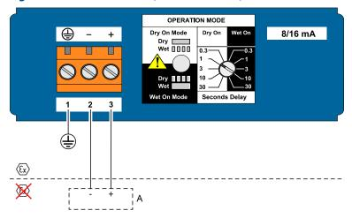
A. A certified intrinsically safe isolating amplifier to IEC 60947-5-6
