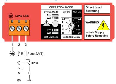
R = External load (must be fitted)
