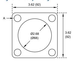
A. 4 off Ø0.55 (Ø14) holes equi-spaced on 3.62 (92) PCD
