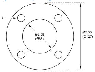
A. 4 off Ø0.55 (Ø14) holes equi-spaced on 3.97 (98.4) PCD
