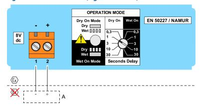
A. A certified intrinsically safe isolating amplifier to IEC 60947-5-6
