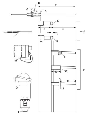
Figure 16: Individual Components of a Complete Temperature Assembly
