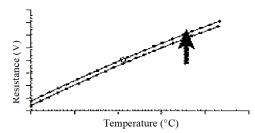
A one-point trim shifts the ideal curve up or down based on the single characterized point.
