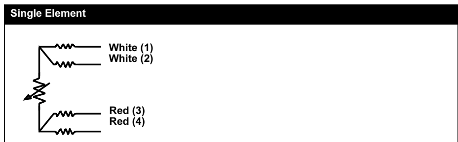
Figure 2-2. Rosemount 68Q, 78 Standard Temperature Range, and 58C RTD Sensor Lead Wire Configurations
