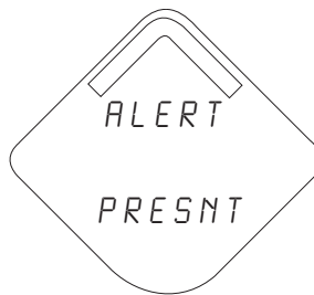
Alert Screen - at least one alert is present - this screen will not display if no alerts are present
