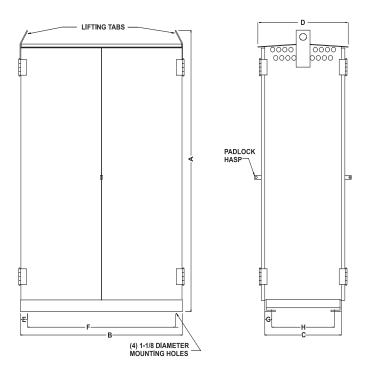
These tamper proof, lockable housings constructed of 12 gauge (.104") steel and rigid angle provide relief from direct sun rays as well as preventing unauthorized tampering. The units have swing out doors with stainless steel hinges for easy access and cylinder change out.
