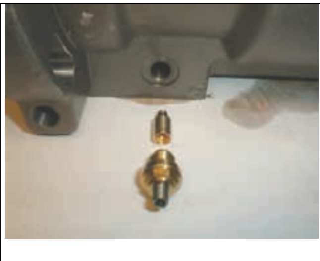
Figure 15: Crossover Valve and Seat Removed
