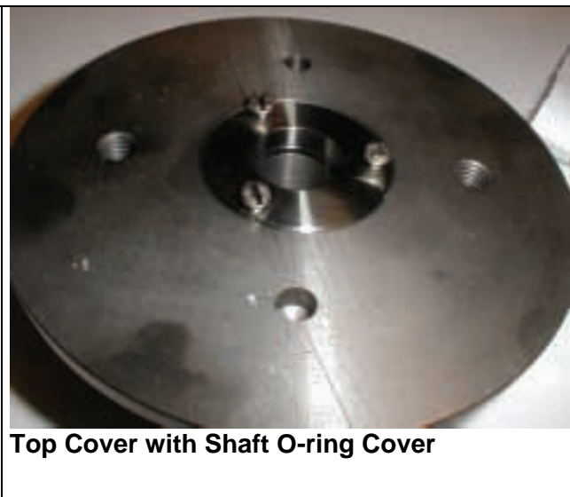
Figure 24: Installing the Shaft O-ring Cover
