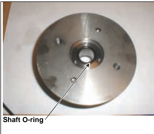
Figure 23: Installing the Shaft O-ring
