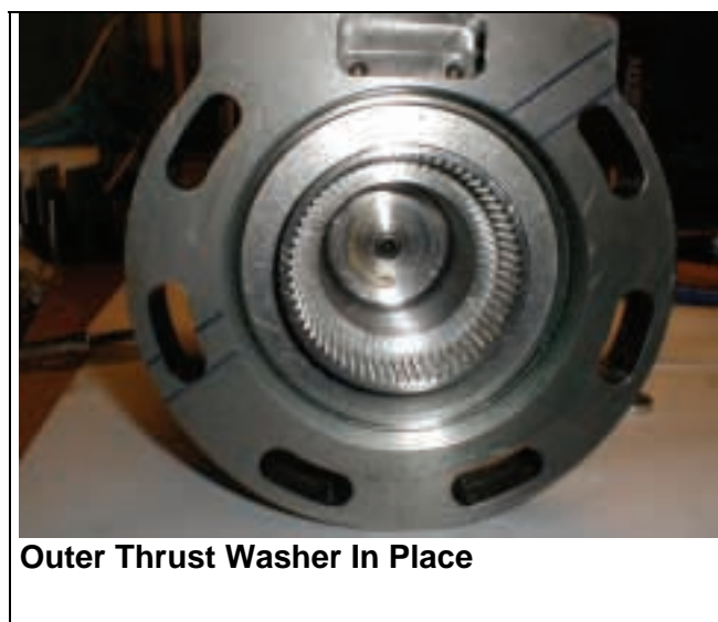
Figure 48: Completed Thrust Bearing Installation
