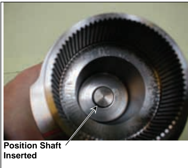
Figure 39: Position Shaft and Spline Shaft
