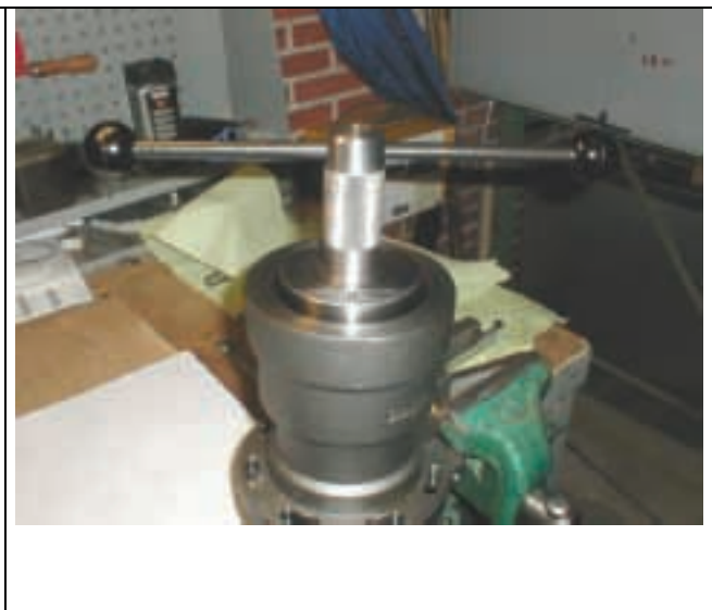
Figure 11: Piston Removal Tool
