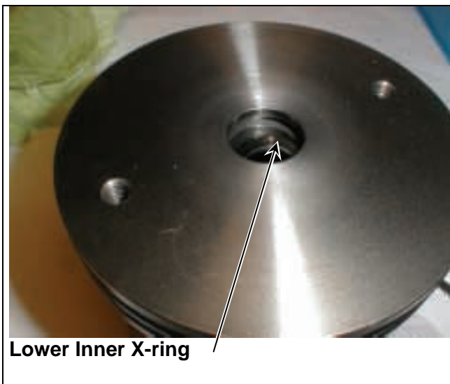
Figure 19: Installing Lower Inner X-ring
