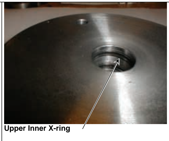
Figure 20: Installing the Upper Inner X-ring
