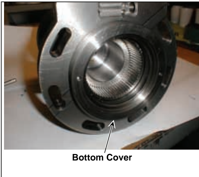
Figure 49: Installing Bottom Cover
