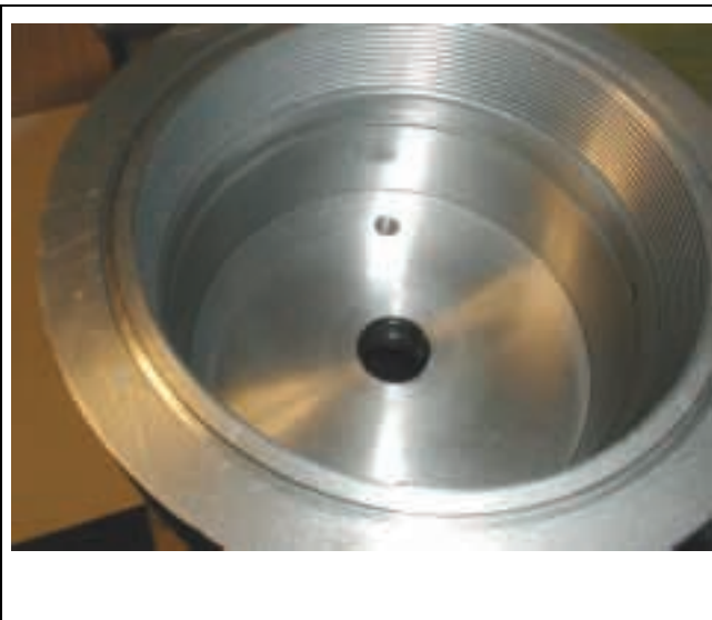
Figure 35: Piston Shown Installed
