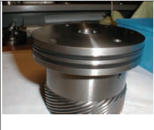
Figure 13: Piston Removed From Cylinder
