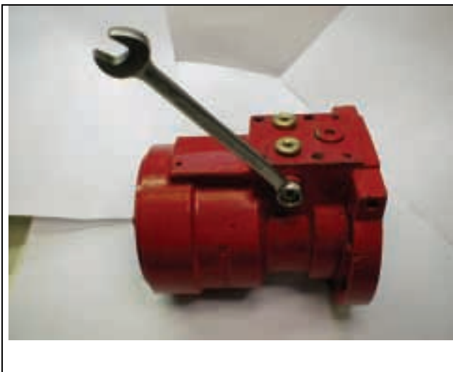
Figure 14: Removal of Crossover Valve
