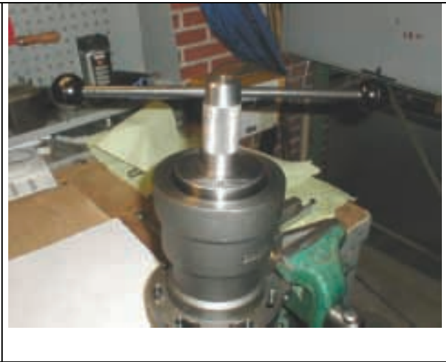
Figure 34: Installation Tool for Piston
