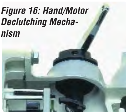
Figure 17: Hand/Auto Declutch Lever
