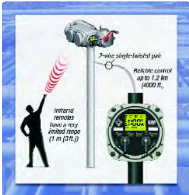
Figure 3: Remote Display Module (RDM) (Patent Pending)
