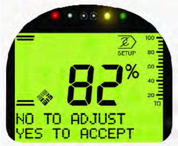
TEC2000 ICONOTEXT DISPLAY showing actuator in SETUP mode and valve 82% OPEN.
