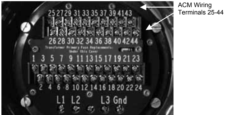
Figure 3-10 ACM Wiring Connections
