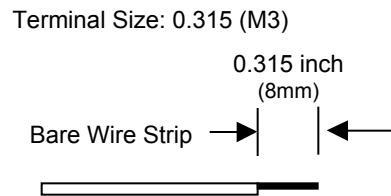
Figure 3-3 Power Terminal Connections
