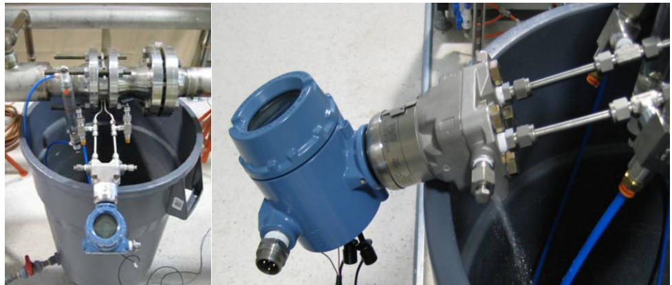
Figure 2 – Controlled Impulse Line Leak Test Setup
