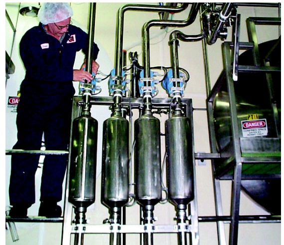
Direct mass measurement of products flowing through Micro Motion 3A authorized T-Series meters has helped to improve first-pass yields at Perry's by 15%
