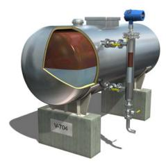
Submerged probe interface applications
