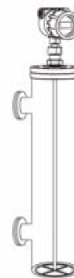
A centering disk helps to keep the probe away from the pipe walls. It is recommended for single rigid probes. Its applicability with long flexible probes is more limited.
