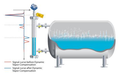
The figure illustrates the radar signal curve before and after vapor compensation. Without compensation, the surface pulse appears to be beyond the actual level. After compensation the surface appears at the correct surface level point.
