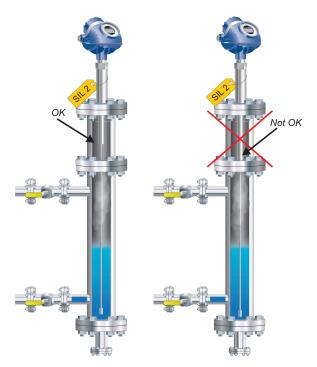
The spool piece needs to be at least 2-in. (50 mm) longer or shorter. For a spool piece with the Dynamic Vapor Compensation integrated still pipe vapor probe, this is not a requirement.
