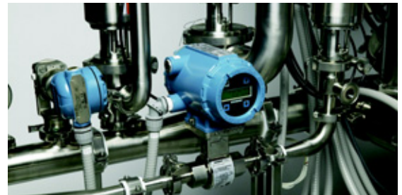
The Rosemount 8721 Hygienic Magmeter Installed
