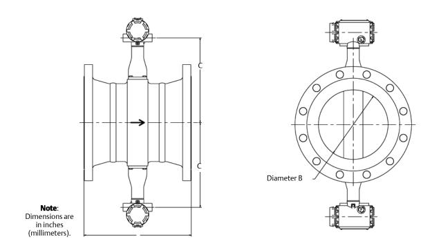
Table A-13. Vortex Dual-Sensor Style Flowmeter (6- through 12-in./100 through 300 mm Line Sizes)
