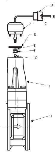
A.? NPT conduit adapter or cable gland (supplied by customer)
