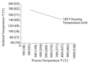
Meter and pipe insulated with 3 inches of ceramic fiber insulation. Horizontal Pipe and Vertical meter position.
