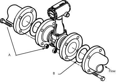
Figure 3-13. Flanged-Style Flowmeter Installation
