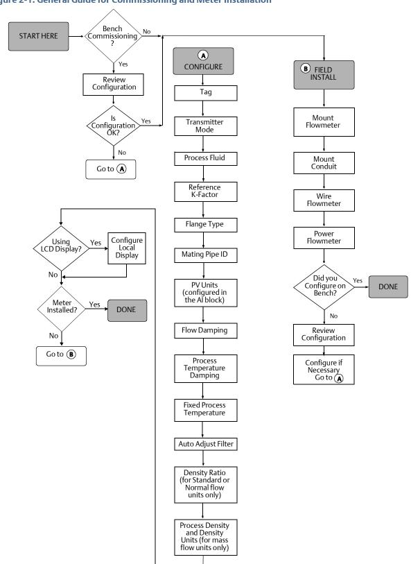
Figure 2-1. General Guide for Commissioning and Meter Installation
