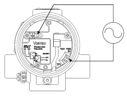
Figure C-10. Test Frequency Input Using the Ground Tab
