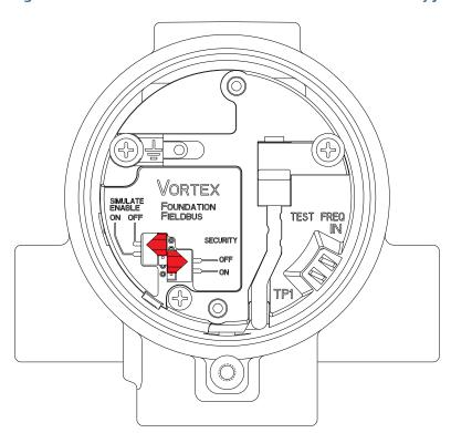
Figure 3-19. Fieldbus Simulate Enable and Transmitter Security Jumpers
