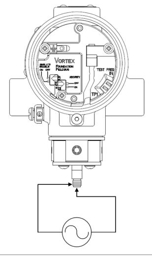
Figure C-12. Using Sensor Header with External Frequency Source
