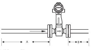
A. 35 diameters (D) upstream B. 10 diameters (D) downstream
