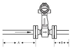
A. 10 diameters (D) upstream B. 5 diameters (D) upstream
