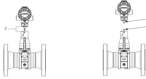
A. Sensor cable nut—SMA connector
