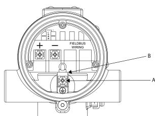
Figure 3-16. Internal Ground Screw Connection
