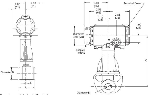
Dimensions are in inches (millimeters). Electronics housing may be rotated in 90 degree increments.
