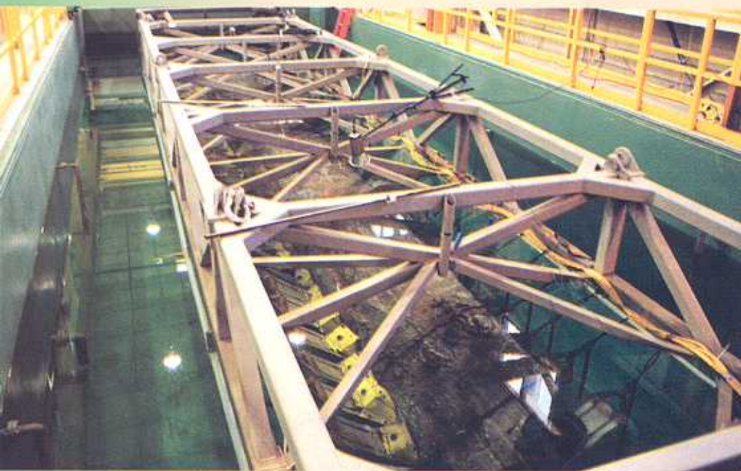
The H.L. Hunley immersed in a large tank filled with an electrolyte solution of water and sodium hydroxide, which draws the chlorides out of the metal.
