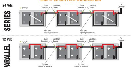
Note: Maximum current is 10 A. For systems over 150 W, the 24 V dc configuration must be used.
