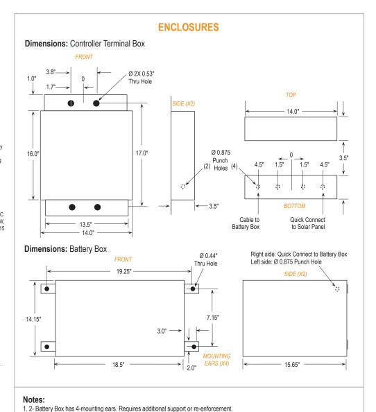
2. Battery Box has two punch holes available (1 each side); Controller Terminal Box has 4 punch holes available (2 bottom/2 each side).
