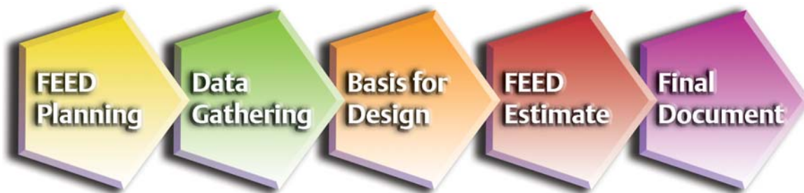
Emerson FEED Work Process
