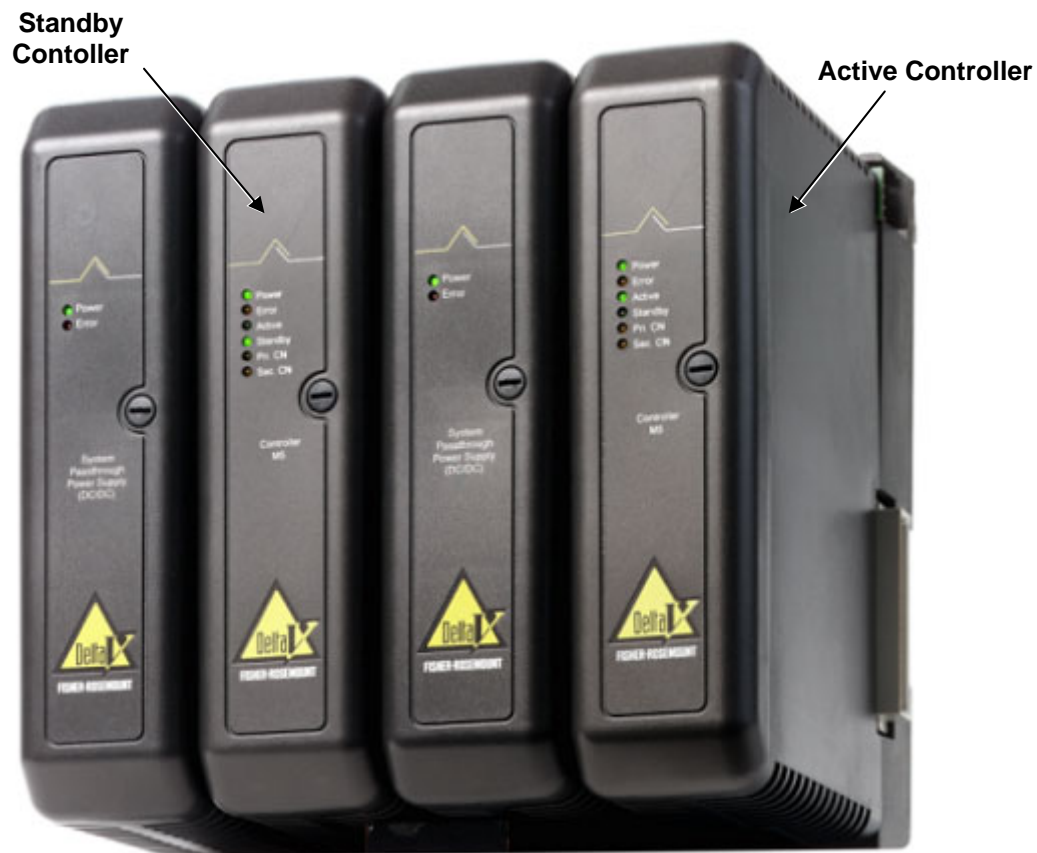
Figure 1. Redundant controller pair
