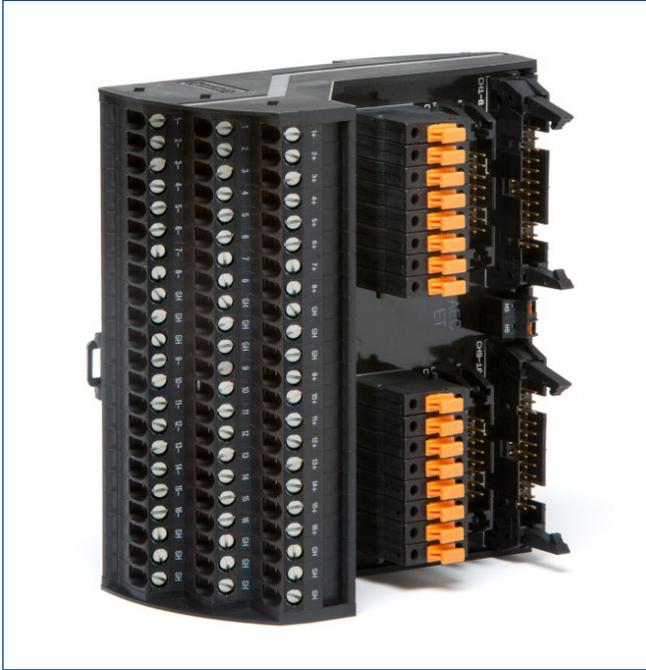
The AI/AO Plus Mass Connection Board connects to the **new S-series Plus** (simplex or redundant) **AI, 16 Channel and AO, 16 Channel** cards by using either two ribbon cables with 24-Pin connectors or the 48-Pin special Round Ribbon Cable, which is required if the distance is longer than 3m.
