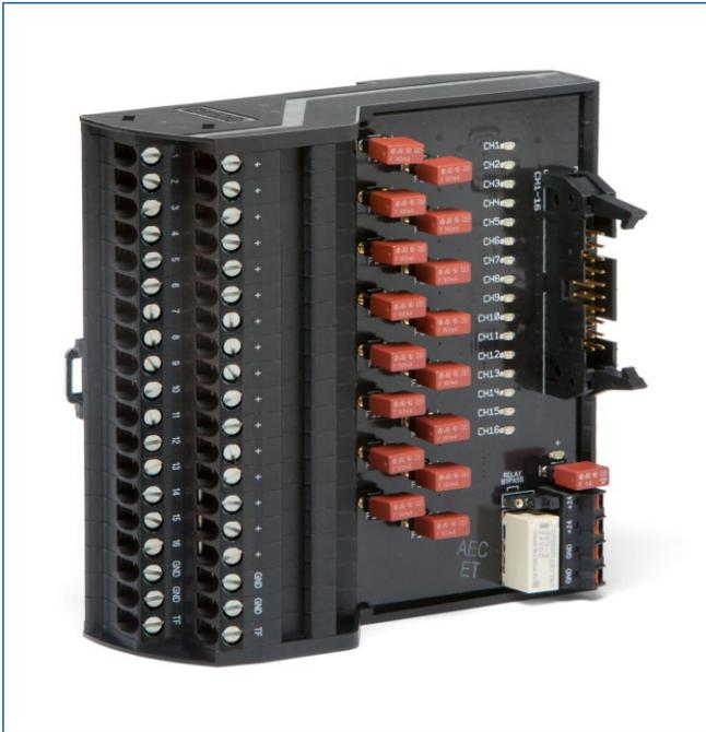
The DI Plus Mass Connection Solution (set of two boards) connects to the **new redundant S-series Plus DI, 32 Channel, 24 VDC, Dry Contact cards** by using either two ribbon cables with 20-Pin connectors or two of the 20-Pin standard Round Ribbon Cable, which is required if the distance is longer than 3m.
