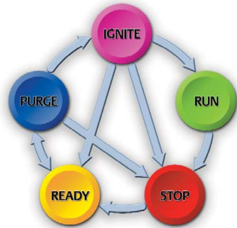
The different states and transitions for a burner are represented by a state transition diagram in the DeltaV SIS system.
