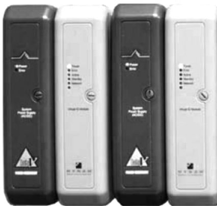
Redundant Virtual I/O Modules providing an Ethernet Network Gateway for a Logic Controller
