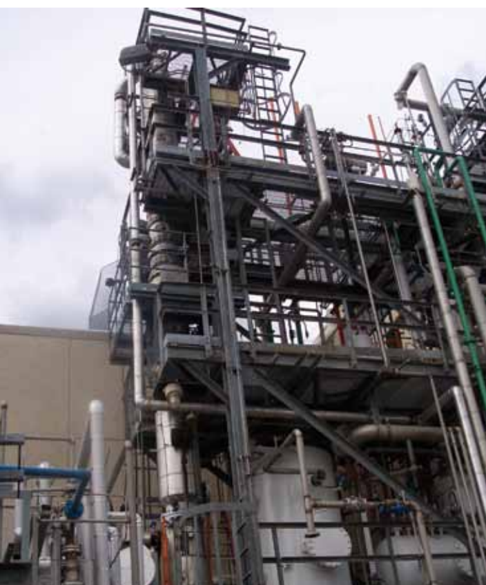
Researchers at the University of Texas at Austin have demonstrated closed-loop control of a distillation column using wireless, with performance virtually undistinguishable from that of wired transmitters.
