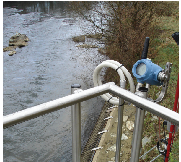
Emerson's Smart Wireless solution monitors river water temperature at the Lenzing Fibers mill.
