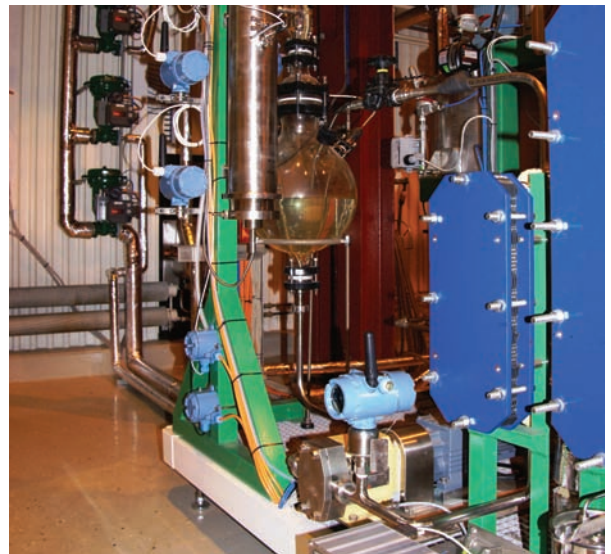
Nine Rosemount wireless pressure transmitters and seven Rosemount wireless temperature transmitters have been installed.
