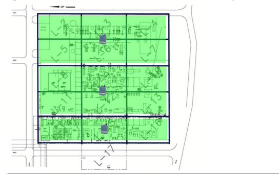
Figure 6-3. Process with Three WirelessHART Networks and Good Gateway Placement
