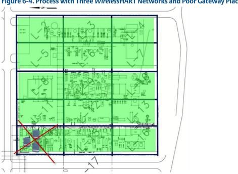
Figure 6-4. Process with Three WirelessHART Networks and Poor Gateway Placement
