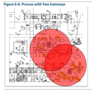
If a wireless device requires update rates faster than two seconds or is used for control and does not meet the "Rule of Maximum Distance", consider adding a Gateway as shown in Figure 6-8 or moving the existing Gateway closer to the wireless device. If the process control loop is tolerant of latency, or if it was previously a form of manual control, it may be acceptable to have devices further from the Gateway.
