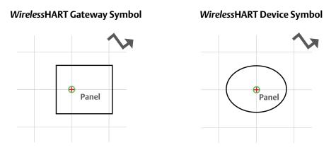
*Wireless*HART devices can be connected to a *Wireless*HART Gateway using the User Defined Field. This type of drawing does not show the path through the *Wireless*HART network, but does show the relationship of the *Wireless*HART device and the *Wireless*HART Gateway; Figure 13-7 is an example from the ISA-5.1.
