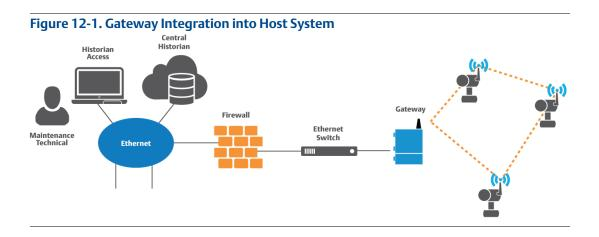
For *Wireless*HART networks that support users in different roles, the potential exists for each end user to have their own application for collecting and analyzing data. For users who manually collect data, *Wireless*HART provides the missing piece to automation.
