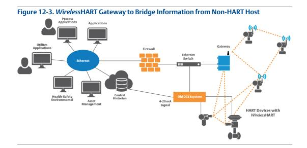
A key output from working with host system administrators is an integration strategy to incorporate a plant-wide wireless infrastructure. If doing a small application, a key output is the physical locations of where to connect the Gateways. These will be needed for the network design process.
