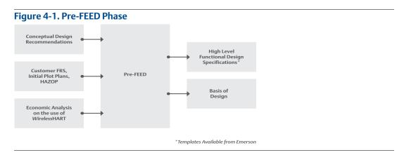
An integrated approach should be used for incorporating wireless into a project. Wireless should be merged with wired technology in the project procedures. It is essential to use the right field device technology for the right application. New end user communities may be added as the cost advantages of wireless expand applications during the FEED process.
