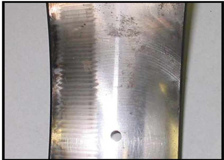
Figure 12. Defective bearing (fluting) from Pulverizer exhaust fan where data presented in Figures 10 and 11 were acquired.
