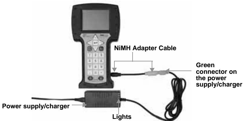
Figure 2. NiMH Adapter Cable used to charge the NiMH Battery Pack
