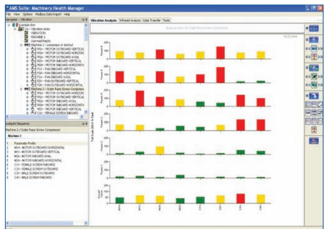
Quickly determine the status of a machine with the Parameter Status Profile.
