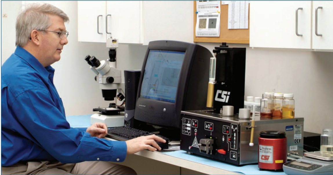
The CSI 5200 is part of a complete minilab system that provides comprehensive oil analysis results.
