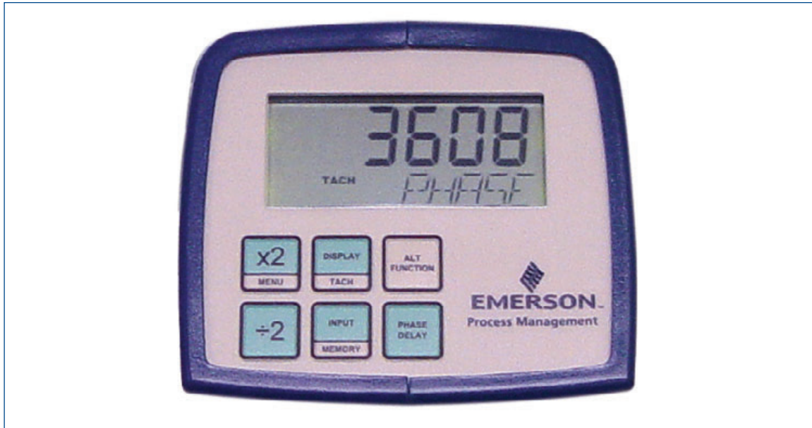
User interface consists of an easy-to-read digital display of RPM and mode with simple keypad buttons for selecting different modes, operations, or views.
