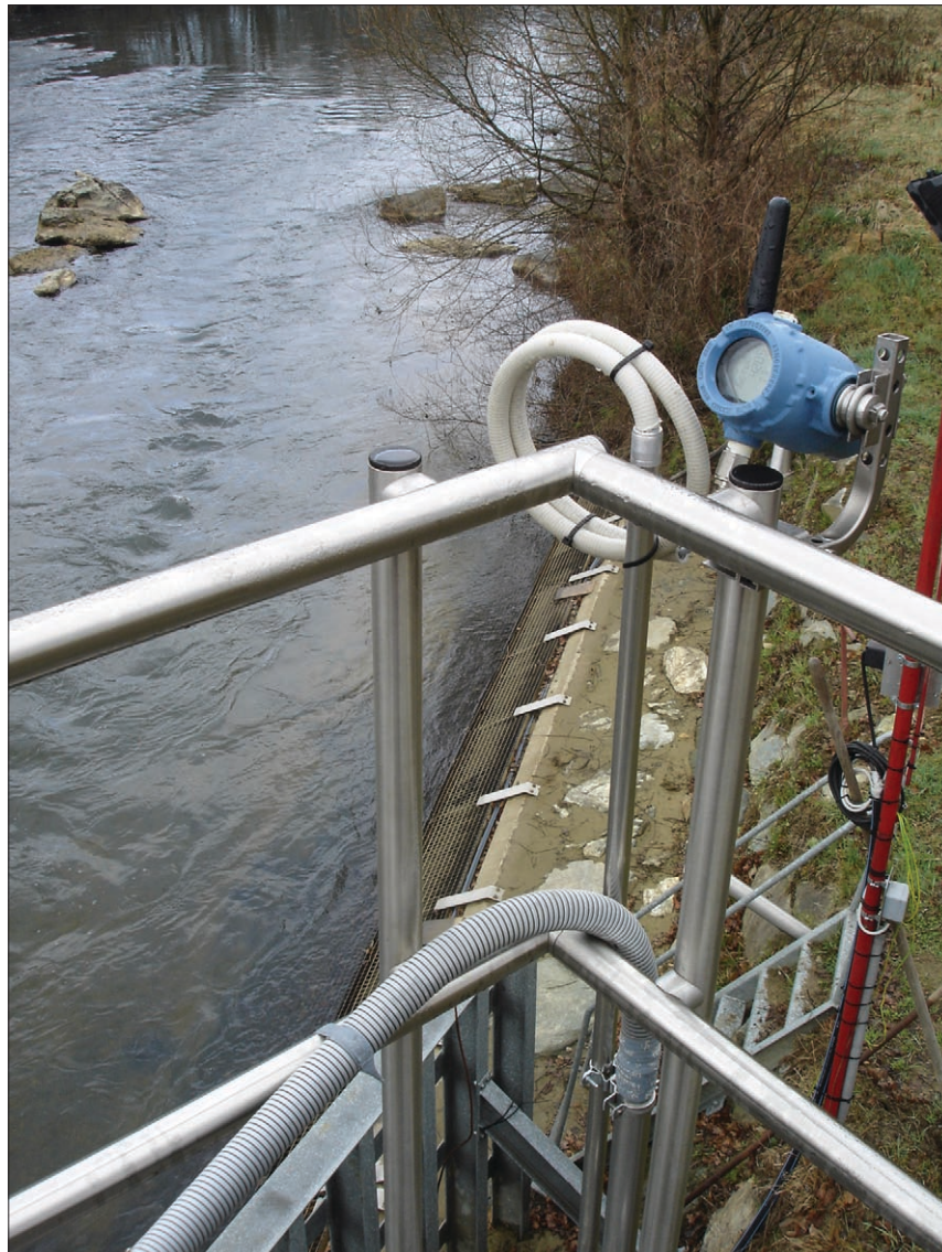
Fig. 1. The temperature of the water extracted from the river is transmitted wirelessly to a Smart Wireless gateway.
