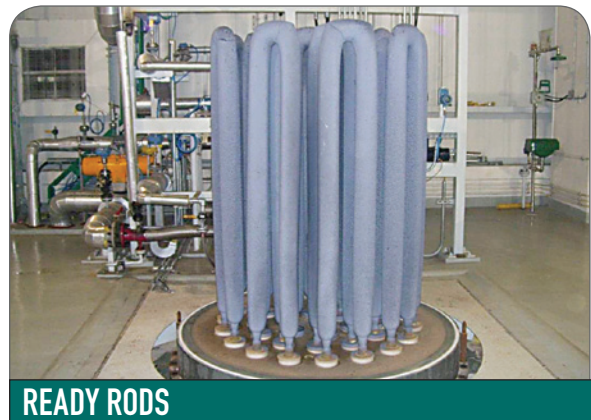
READY RODS Figure 3: Only 24 months after breaking ground, Production Line 1 at LDK Solar's polysilicon plant began producing product, such as these polysilicon rods ready for harvest, on Sept. 8, 2009.
