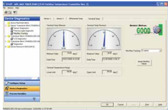
Dial indicators for visual display of transmitter temperature extremes.
