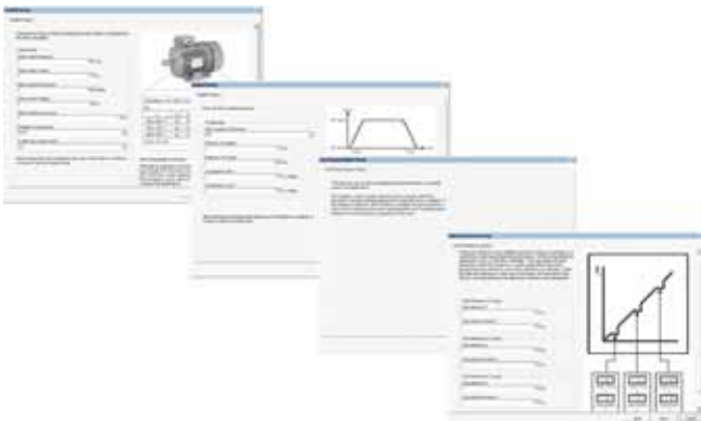
For setup, driver-manufacturer-created wizards with help text and illustrations guide the technician step-by-step
