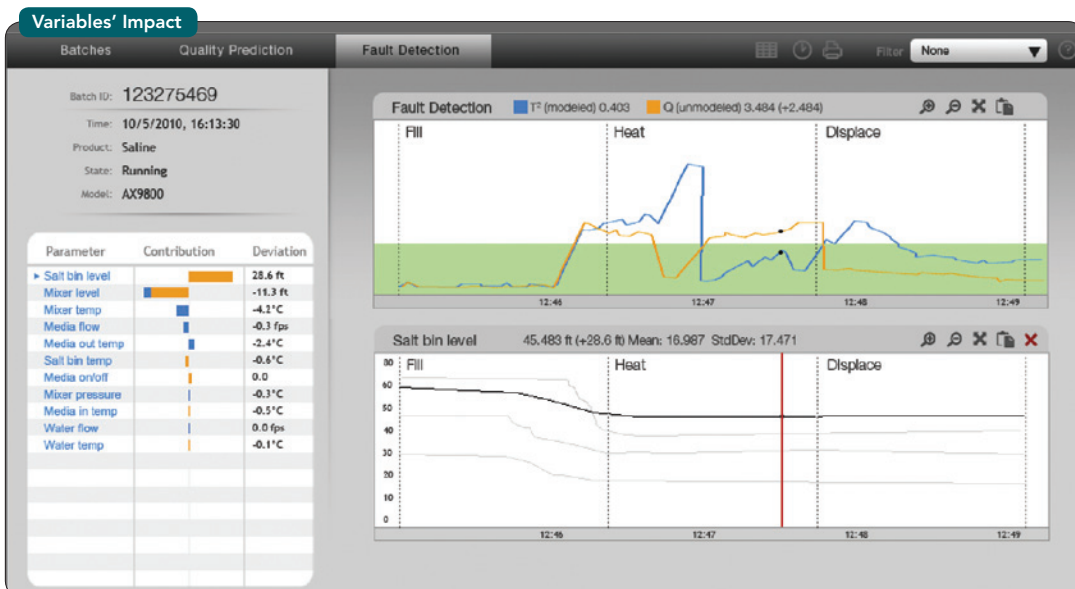
Figure 4. Operators can view the contribution of all variables related to a fault.
